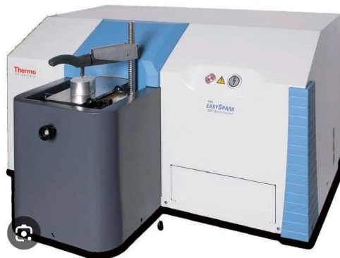
Spectrometer for chemical composition
